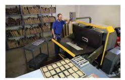
PRECISION DIE CUTTING Mar-Tek has two precision clam shell presses, each capable of cutting materials within tolerances of +/- .010".
